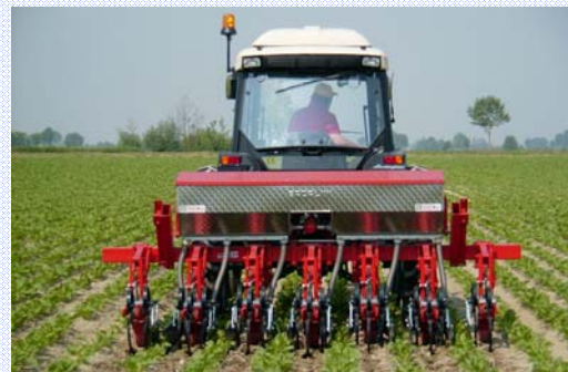
ON THE LEFT: MACHINE FOR WORK ON MAIZE OR SUNFLOWERS WITH HYDRAULIC FOLDING FRAME TO 2,45 METERS
