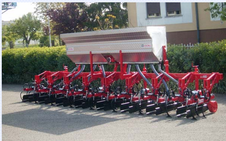
CULTIVATOR FOR WORK ON MAIZE WITH FERTILIZER DISTRIBUTOR
