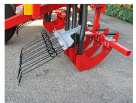
SET TO LAY UNDERGROUND FERTILIZER
