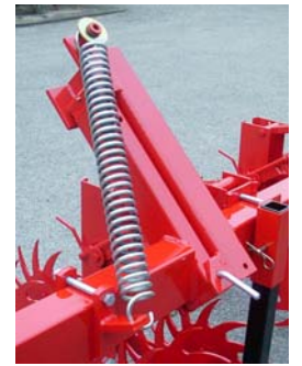
Turnover hinge with spring to facilitate the mechanical manual closing
