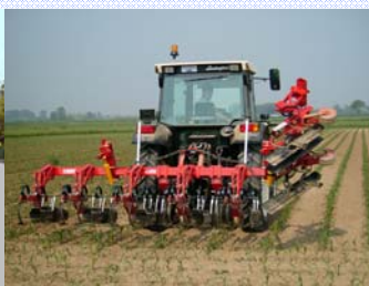
ON THE LEFT: MACHINE FOR WORK ON MAIZE OR SUNFLOWERS WITH HYDRAULIC FOLDING FRAME TO 2,45 METERS
