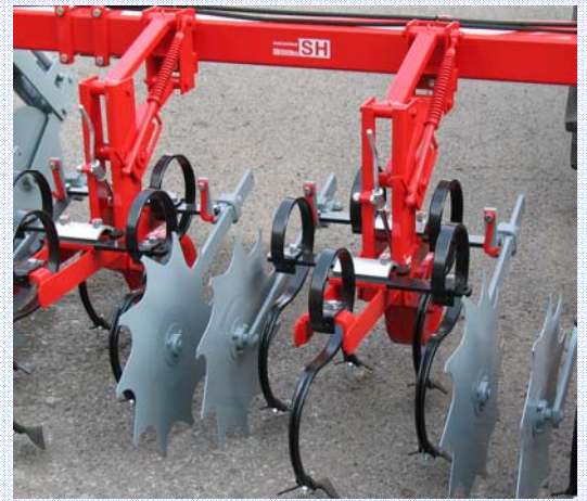
PARALLELOGRAM WITH BUSHING AND LUBRICATOR ON EVERY ARTICULATED JOINT
