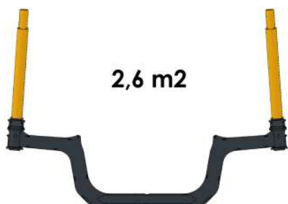
GROUP 2 POLES WITH LOAD AREA EXTENSIONS IN THE OPEN POSITION
