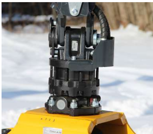
Rotator with hose protection cover
