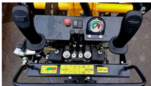
Valve block 4/8 XY control ON-OFF with additional equipment
