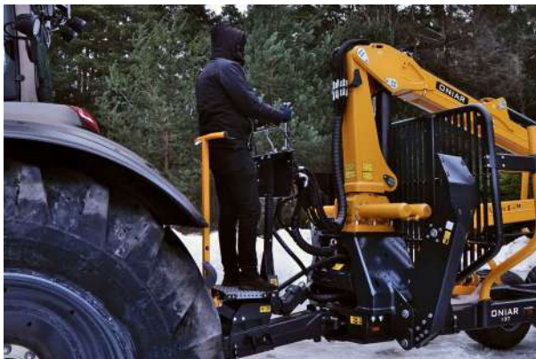
Standing platform for control valve on drawbar with pump connection underneath
