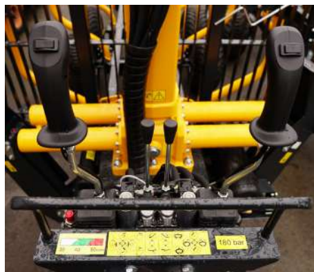
Valve block 4/8 XY control ON-OFF
