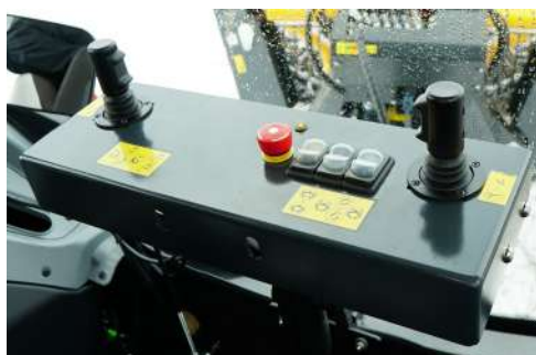
Valve block full electric with mini joysticks FIX / LS
