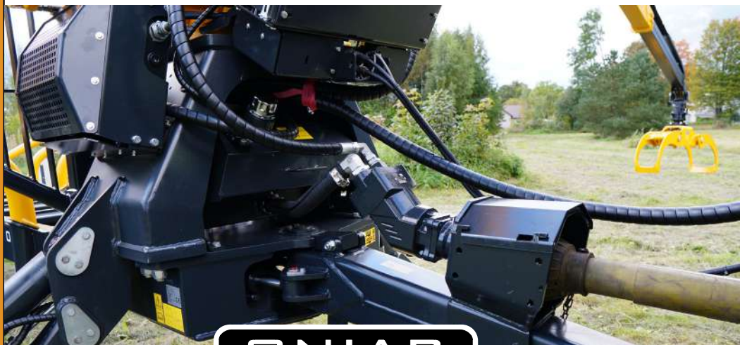
Pistonpump & reductor in PTO
