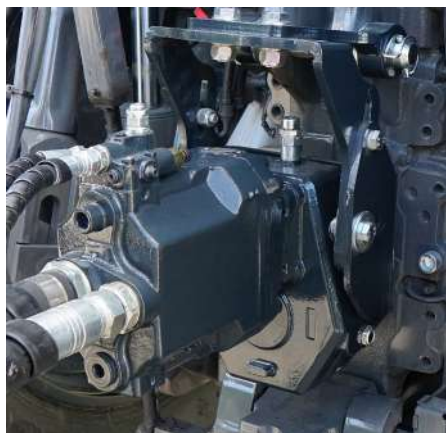
Pistonpump & reductor in PTO
